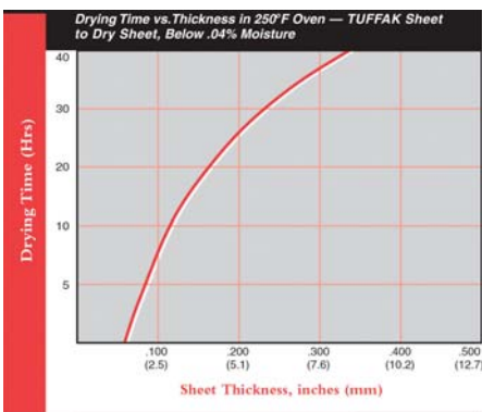
Figure 1. Drying time of Tuffak® polycarbonate sheet vs. thickness in a 250°F oven. The time indicated is that required to achieve 0.04 percent moisture or less.
